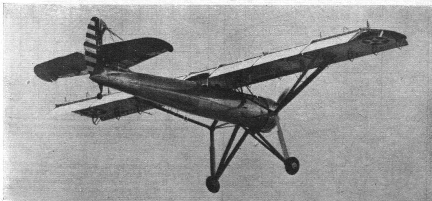
The new Ryan YO-51 light army co-operation machine built to the Fieseler Storch formula. Fully slotted and flapped, it can be operated from extremely small spaces and is enabled to fly very slowly for artillery spotting.
