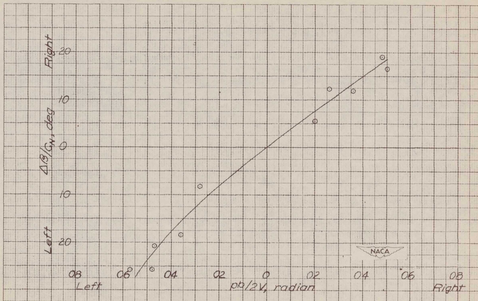
(b) Plot of change in sideslip angle divided by normal force coefficient against maximum pb/2V .
