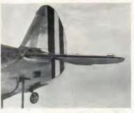
2. Vertical Stabilizer or Fin... This structure is similar to that of the horizontal stabilizer and is attached to it by means of 8 forged aluminum alloy fittings. The skin is of the stressed type, riveted to the webs and bulkheads by means of flush type riveting from the leading edge aft to web No. 1. The remainder of the riveting is of the modified brazier head type.
