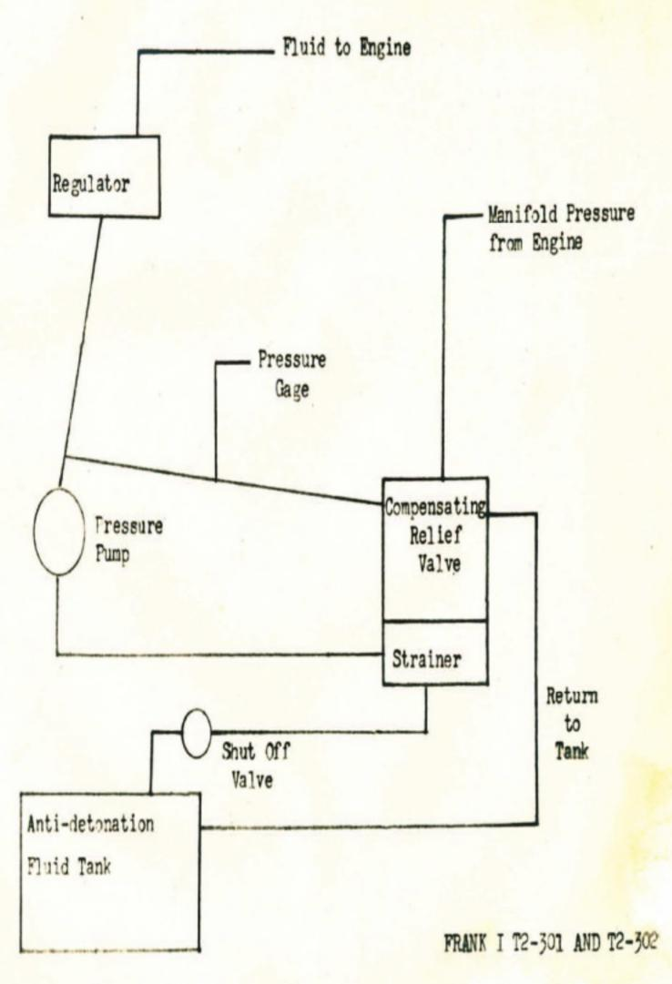
ANTI-DEFORATION INJECTION WISTEM
