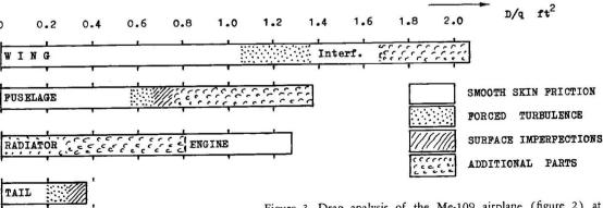
Figure 3. Drag analysis of the Me-109 airplane (figure 2) at  $V_{max}=610$  km/h,  $C_{\c L}=0.21$  and M=0.55.
